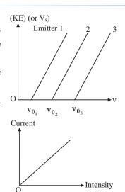
5. If the collector potential with respect to the emitter is reduced to zero, current does not reduce to zero. If the collector potential is made negative with respect to the emitter and then increased, the current decreases. At a particular negative potential (V<sub>s</sub>), the photoelectric current becomes zero. This potential is called stopping potential.
